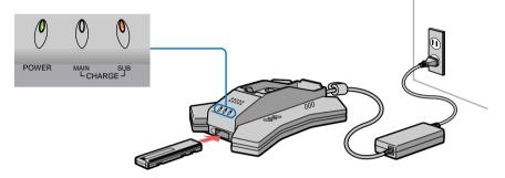
When charging AIBO and the extra battery at the same time The MAIN indicator lights up in orange. When charging is completed, it will light up in green.
